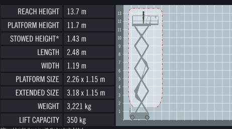
**ELECTRIC POWERED** Perfect for indoor applications **NON MARKING TYRES** Prevents marking to finished floors
